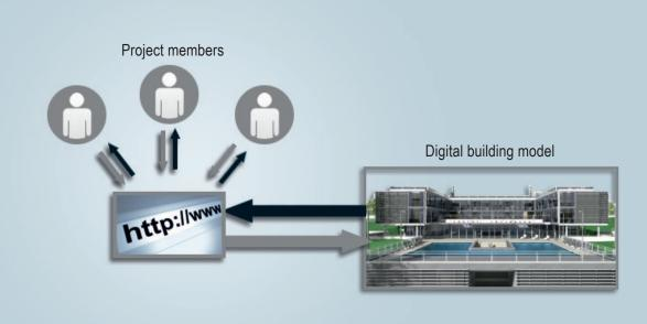
AllplanWorkgroup Manager assumes the organization of CAD work stations in local networks (LAN) as well as via Internet. It creates clear synergy effects in medium-sized and large planning and construction firms. Work at an individual network work station is just as simple as work at a normal individual station. The main advantage of the Workgroup Manager is that project data and users and their access options can be managed centrally. The entire access to data across the network is transparent.
